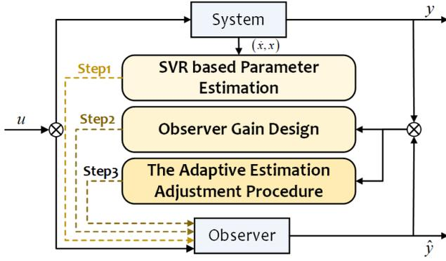
Fig. 1: The design of proposed estimator structure
