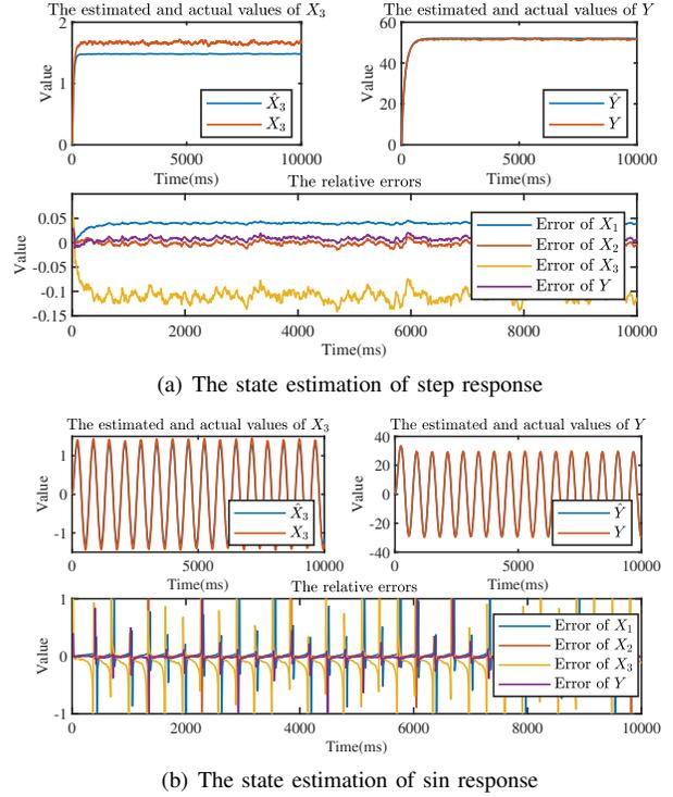
Fig. 2: The state estimation without adjustment procedure of the performance of the model. We get  $\hat{\mathbf{A}}_0$  as  $\hat{\mathbf{A}}_0 = \text{diag}\{-4.78, -10.03, -16.95\}$ .
