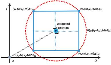
Fig. 2. After time slot  $T_{12}$ ,  $R_j$  lies in the uncertainty area, i.e., the circle region  $\delta(p_i(t_1 + T_{12}), M\Delta T_{02})$ . 'O' is the estimated position of  $R_j$  when  $R_i$  finishes obstacle-avoidance at  $t_1$ .
