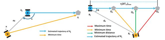
(a)  $\alpha > \alpha_0$ : if  $v_i^{max} \geq v_j^c$ ,  $R_i$  is able to catch up with  $R_j$  at estimated point short for  $R_i$ , and the velocity constraints is loosen.
