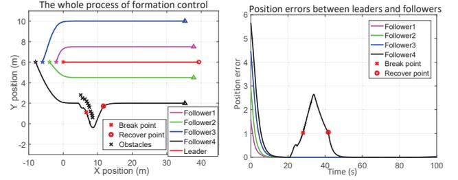
(c) Follower 4 loses connectivity with (d) Follower's errors between real position and desired position
