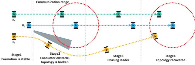
Fig. 1. The whole process of the scenario we focus on in this paper, which can be divided into 4 stages.  $R_j$  is the leader,  $R_i$  and  $R_k$  are  $R_j$ 's two followers. When  $R_i$  loses communication with  $R_j$ , it will recover the topology based on the proposed motion estimation and control strategy.
